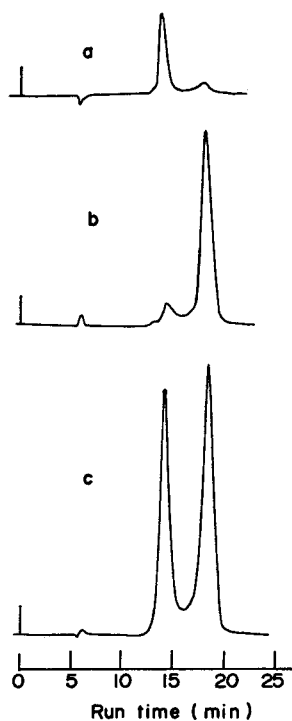
Fig. 4. Separation of the anomers of D-glucose; (a) \alpha -anomer and (b) \beta -anomer injected within 30 min after dissolution and (c) \alpha -anomer after equilibration in 80% ethanol. Conditions as in Fig. 1.
